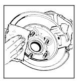
Remove any rust or dirt from the wheel bolts, mounting surfaces and spare wheel. 7. Install the compact spare tire.
